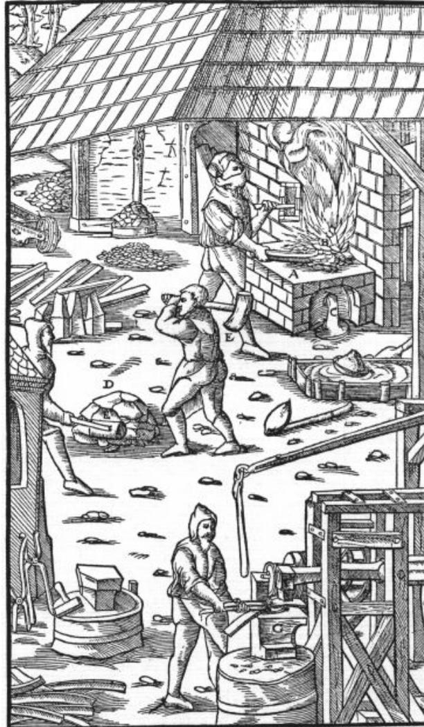
A—HEARTH. B—HEAP. C—SLAG-VENT. D—IRON MASS. E—WOODEN MALLETS.
